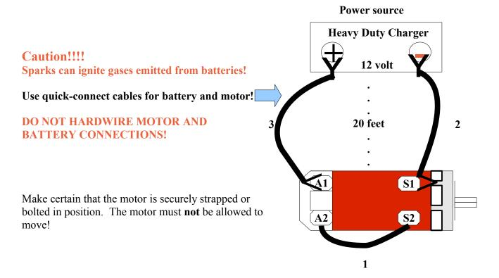
If a battery is used instead of a charger, the battery must be at least 20 feet away from the motor in a well ventilated area or preferably outside of the building!
