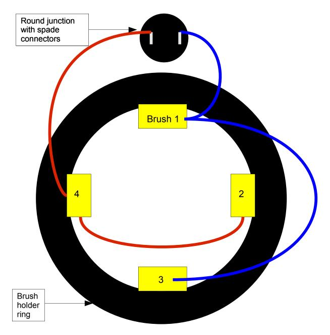
Circuit is completed when brush sensor wire 1 or 3 AND brush wear sensor 2 OR 4 make contact with the armature. Armature voltage will then be present at the connector.
