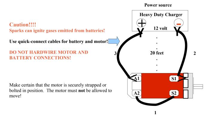
If a battery is used instead of a charger, the battery must be at least 20 feet away from the motor in a well ventilated area or preferably outside of the building!
