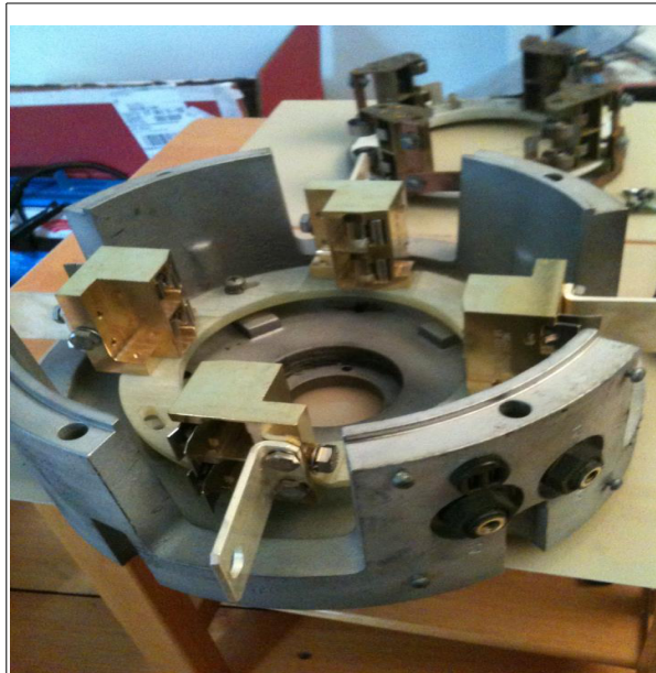
Illustration 37: Ultra High Performance Brush Rigging from Helwig-Carbon
