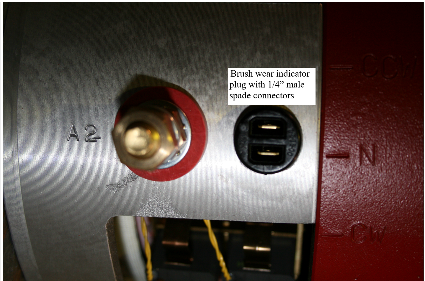
Illustration 30: Brush Wear Indicator Plug
