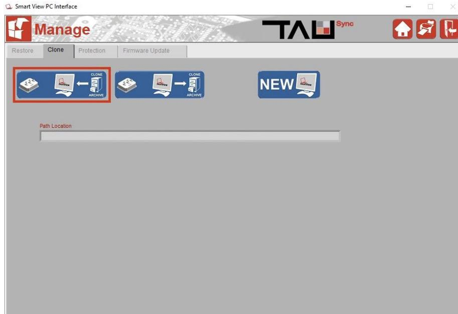
**Manage – Clone – To Controller:** To load a Clone file to your computer, navigate to the file that you saved on your computer. Saving a clone on your desktop is an easily accessible option, then you can click the Desktop Icon to access .clon type files saved on your desktop. Select the clone file you wish to install on your controller. Then click OK.
